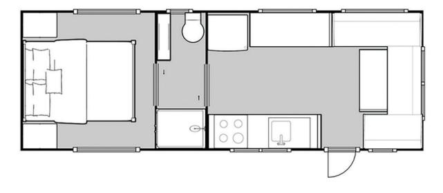
CARAVAN LENGTH: 23' / 7m OVERALL LENGTH: 8.6m HEIGHT: 2.9m WIDTH: 2.45M WEIGHT: 2700kg (approx.) PAYLOAD: 800kg (approx.) ATM: 3500kg
