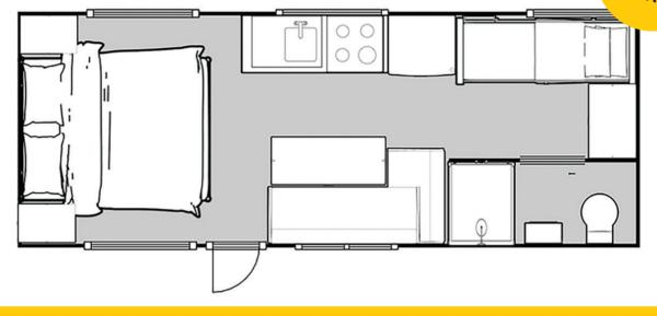
CARAVAN LENGTH: 21' / 6.4m OVERALL LENGTH: 8m HEIGHT: 2.9m WIDTH: 2.45M WEIGHT: 2500kg (approx.) PAYLOAD: 700kg (approx.) ATM: 3200kg
