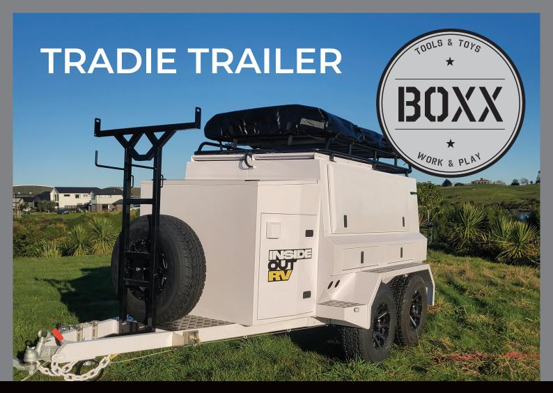
OVERALL LENGTH: 4500mm BODY LENGTH: 3100mm HEIGHT: 2100mm WIDTH: 2200mm WEIGHT: 1100kg (approx.) PAYLOAD: 1900kg (approx.) ATM: 3000kg
