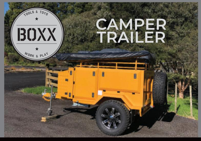
OVERALL LENGTH: 3700mm BODY LENGTH: 2530mm HEIGHT: 2000mm WIDTH: 1850mm WEIGHT: 690kg (approx.) PAYLOAD: 1110kg (approx.) ATM: 2000kg
